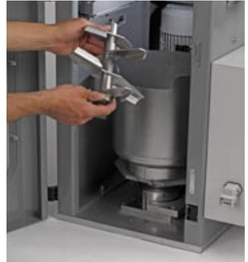
The **loss-in-weight function** is included, thus making the mechanical construction particularly compact. The mixer positioned on the weigh pan is used as a gravimetric hopper for the calculation of the extruder's output, allowing thus detection of any minimum variation. The system is able to rapidly operate and keep the required production parameters constant.
