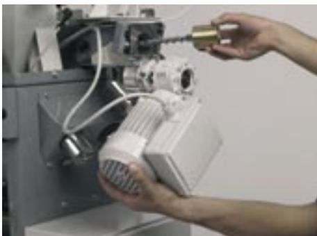
All models are equipped with pneumatically operated slide gates specifically designed to ensure high reliability for any type of material and dosing augers, ideal for precise dosing.
